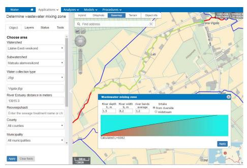
**River-wastewater mixing zone** — Produces diagrams and maps of how wastewater from the shore or rivers mixes and disperses.
