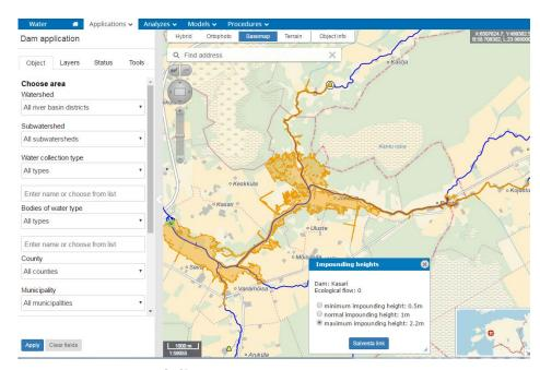
**Dam Impact Modeling**— Enables research on how land is flooded based on the swelling height behind a dam.
