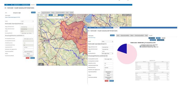
**Estimation Model (Estmodel)**— Calculates and models what the impact to the surrounding environment will be when new structures are built at specific sites.
